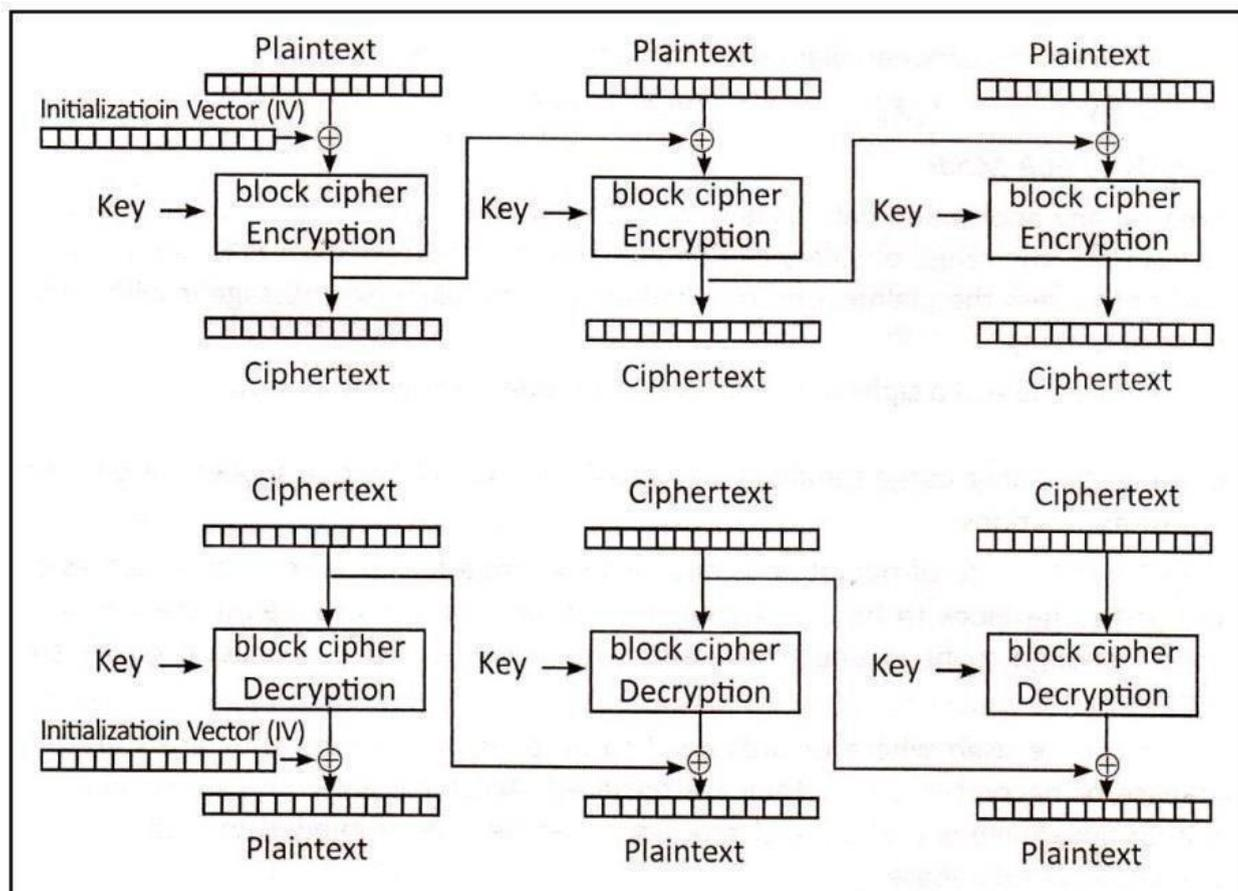
**Fig-1: Encryption & Decryption Process of C.B.C**
