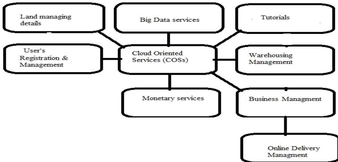
The architecture for Cloud Oriented Services is in the figure, which contains various modules as services for the Indoor farm users and for their farming. Basically the COSs monitors all the other modules. Each and every modules are independent in their operations but to actively participate it needs the COSs web portal. It is useful service for gaining knowledge, crops security, business management and many more services, which can be made use of.
