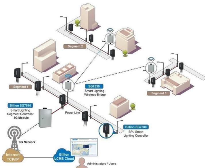
**Fig.2 Data flow diagram for smart street lights.**
