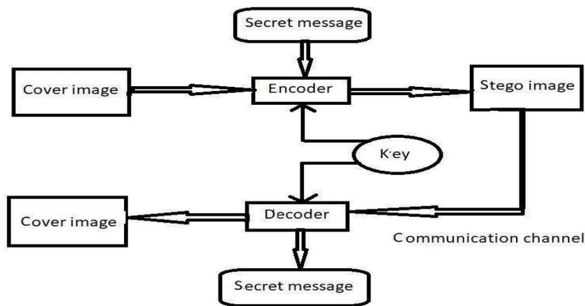
Figure 1.2: Block Diagram of combined Cryptography and Steganography Process
